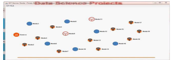
Figure 12: Attack identified at node 9 and node 11 and by pass the route and sends the data to the destination
